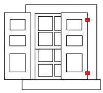
with a gudgeon. The pintle half is mounted to the window with the pintle pointing up. Offset is measured from the shutter face to the center of the pin.
