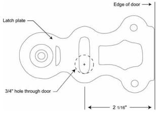
2. With the latch plate in its desired position, mark the center location of the 3/4" hole as shown. The hole should be centered horizontally in the oval slot and 3/8" up from the bottom of the slot. Check to see that the hole is also 2 1/16" from the edge of the door. Drill the 3/4" diameter hole through the door.
