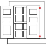
the pintle pointing up. Offset is measured from the shutter face to the center of the pin.
