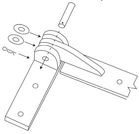
hinge pin and separate the hinge from the base. Now screw each base to the house, position the shutter, and install the hinge pin, spacer washers, and hairpin clip in the hole of the hinge pin.
