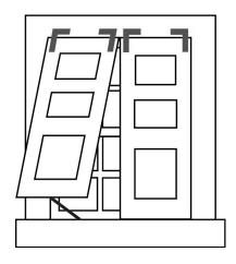
Typically, one hinge is mounted on each side of the outside of shutter at the top as shown above. (Drilling a pilot hole before installing all screws is recommended.) The base is then attached to the hinge by installing the hinge pin as shown below. Use the spacer washers to center the hinge in the base and prevent side-to-side movement. Position the shutter over the window as desired and carefully mark the location of the screw holes for each base. Remove the
