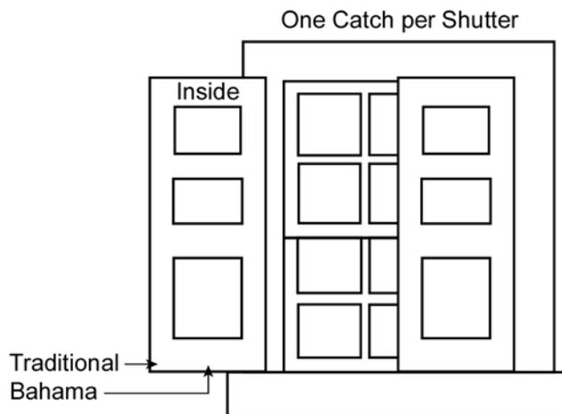
Test fit the catch and make sure it operates properly. Mark the position of the screws and drill a pilot hole before installing the screws. After tightening the screws, make sure the catch operates properly. If needed, now install additional catches in the same way.
