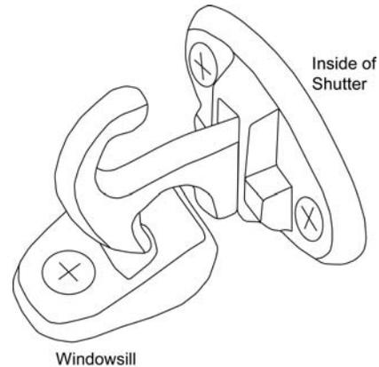
Assemble the catch as shown to the above right. Slide the latch into the mounting base from the back. The hook must point down. You may wish to use tape to temporarily hold the latch into the base so as to more easily position the parts for mounting. The latch and base are mounted to the inside of the shutter at the bottom. The keeper is mounted to the windowsill so that it will engage the latch when the shutter is in the closed position.
