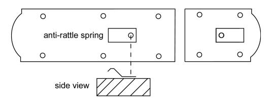
4. Drill 1/16" pilot holes at the locations you marked for the bolt and catch. Place the bolt and catch over the springs and screw them to the shutters. Test the operation.
